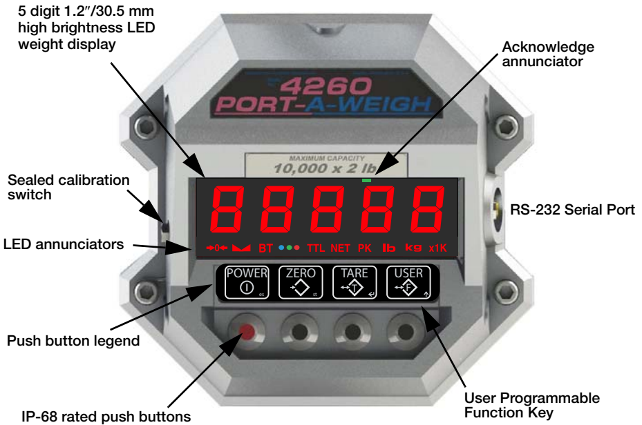
Figure 1-1 MSI-4260 Front Panel
